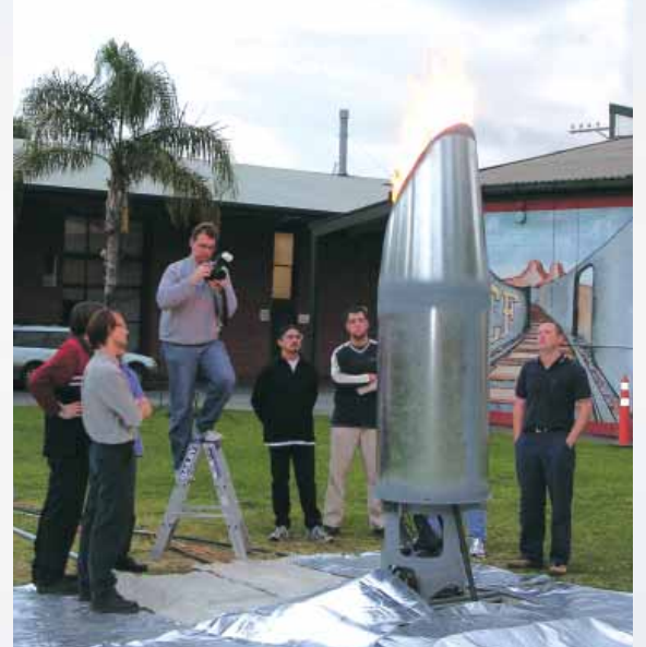
BURNING BRIGHT: the FCT-Combustion/University team tests the main stadium cauldron burner at Thebarton
