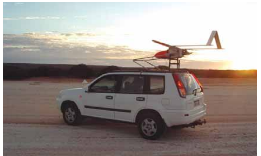
The Unmanned Aerial Vehicle (above) is launched from the roof of a moving car (below)
