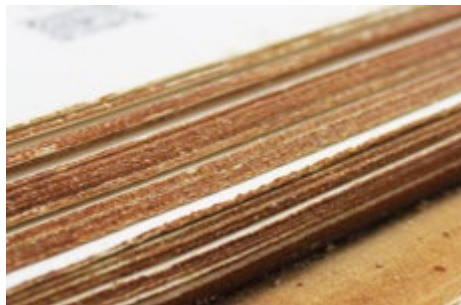
400 pictures of our people: Sketches from 'Punch'. Charles Keene. 1888. Caoutchouc binding, showing typical degradation of the rubber.
