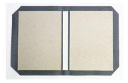
Case construction. A simple template of the cased book cover. The cloth margins would be turned over the boards to complete the construction.
