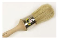
This large Italian round brush is made of natural hog hair bristles and is mounted on a solid wooden handle. Its stiff bristles make it perfect for applying PVA, paste and other cold glues as well as hot hide glues. The large brush is preferred by many binders as it holds enough glue to prepare a cloth cover in one go.
